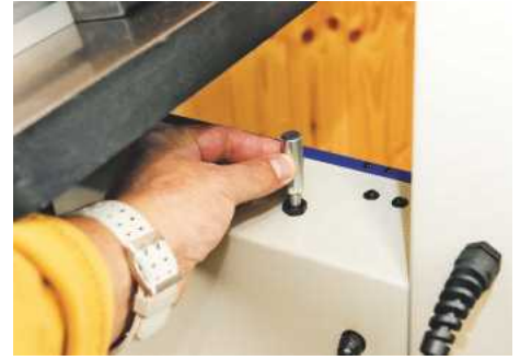
▲ This post allows the table to be set perfectly square to the blade
